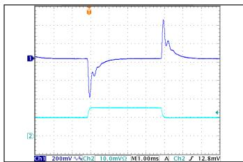
Figure 5: Output voltage response to step-change in load current (50%-75%-50% of lout(max); dI/dt = 0.1 A/µs). Load cap: 1 µF ceramic capacitor. Ch 1: Vout, Ch 2: I = 0.5 A/div.
