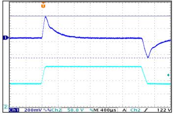
Figure 6: Output voltage response to step-change in input voltage (1V/ms). Load cap: 1 µF ceramic capacitor. Ch 1: Vout, Ch 2: Vin.
