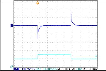
Figure 5: Output voltage response to step-change in load current (50%-75%-50% of lout(max);  $dI/dt = 0.1 \ A/\mu s$ ). Load cap:  $1 \ \mu F$  ceramic and  $15 \ \mu F$  tantalum capacitors. Ch 1: Vout, Ch 2: lout(5.0A/div).
