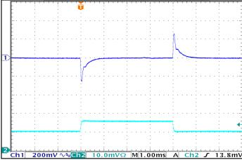
Figure 5: Output voltage response to step-change in load current (50%-75%-50% of Iout(max);  $dI/dt = 0.1 \text{ A/\mu s}$ ). Load cap:  $1 \mu F$  ceramic capacitor. Ch 1: Vout, Ch 2: Iout(1.0A/div).
