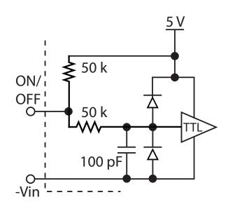
Figure B: Internal ON/OFF pin circuitry
