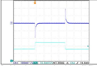
Figure 5: Output voltage response to step-change in load current (50%-75%-50% of lout(max);  $dI/dt = 0.1~A/\mu s$ ). Load cap:  $1~\mu F$  ceramic and  $15~\mu F$  tantalum capacitors. Ch 1: Vout, Ch 2: Iout(1.0A/div).
