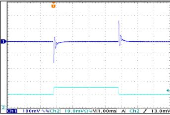
Figure 5: Output voltage response to step-change in load current (50%-75%-50% of Iout(max);  $dI/dt = 0.1~A/\mu s$ ). Load cap:  $1~\mu F$  ceramic and 15  $\mu F$  tantalum capacitors. Ch 1: Vout, Ch 2: Iout(2.0A/div).
